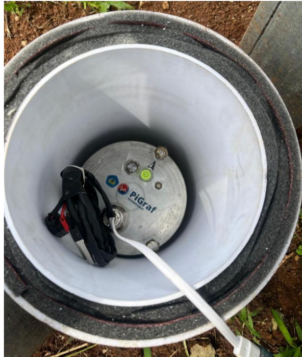
Gambar 17. Casing alat PiGraf
