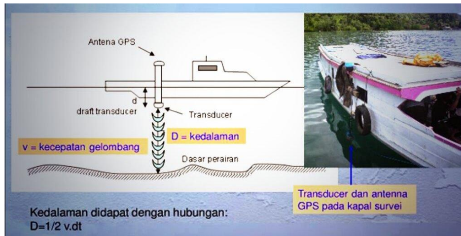
Gambar 4. Prinsip kerja singlebeam echosounder
