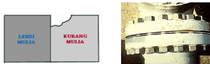
Gambar 2.2. Korosi dwi logam (sumber Priyotomo, 2008)
