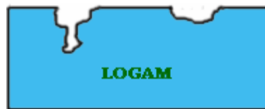
Gambar 2.4. Korosi sumuran ( pitting corrosion ) (sumber Priyotomo, 2008).
