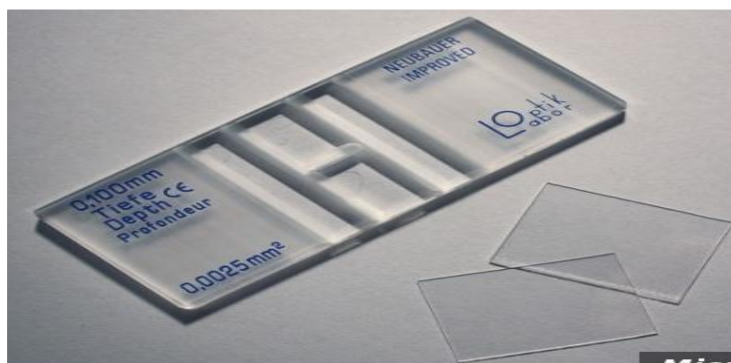
Gambar 5. Haemocytometer Neubauer improved (Caprette, 2007).
