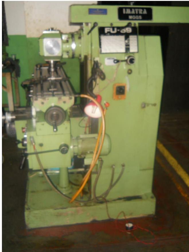
Gambar 3.2. Mesin Frais Horizontal
