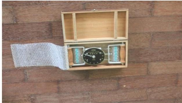
Gambar 8. Pull & Push Dynamometer
