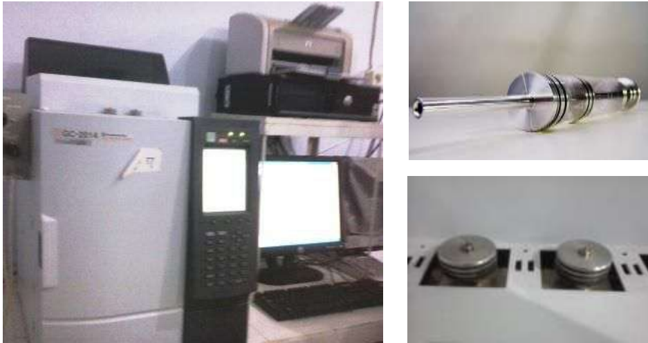
Gambar 3. (a) Gas Chromatography 2014 Shimidzu , (b) Pencadang Gas Pembawa - Siring (c) Lubang injeksi
