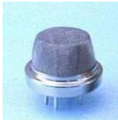
Gambar 2.5 Sensor gas ammonia MQ 137
