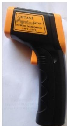
Gambar 3. *Infrared Thermometer*
