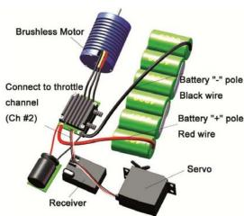
2.1 Turn on the transmitter, set the "EPA/ATV" value of throttle channel to "100%", and <u>disable the "ABS" brake function</u> of your transmitter if it does has this function. If you are using a Futaba transmitter, please set the direction of the throttle channel to "REV"
