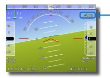
View the strength of the radio signal in the mission planner's flight data screen.
