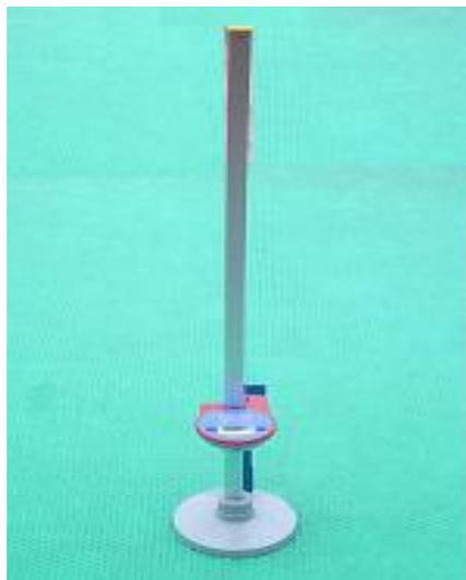
Gambar 6. Trunk Extention Test (digital).
