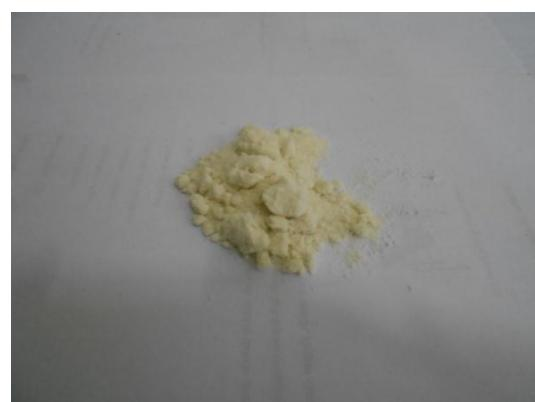
Gambar 21. Serbuk NBR (*Nitrile Butadiene Rubber*)
