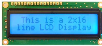
Gambar 2.9 LCD 2x16
