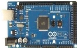
Gambar 2.14 Arduino Mega 2560
