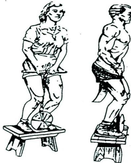
Gambar 9 . Leg Dynamometer
