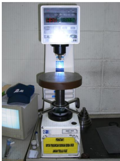
Gambar 32. ( Hardness Tester Future Tech ) di Laboratorium High Quality Control PT. AAI Karawang.
