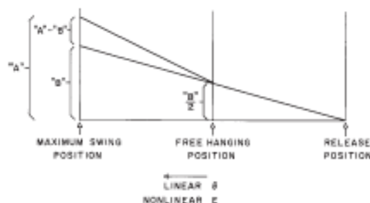
FIG. A1.1 Method of Construction of a Windage and Friction Correction Chart
