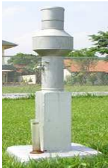
Gambar 2.1. Alat Ukur Curah Hujan (Ombrometer) (Achmadi, 2009)
