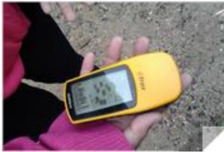
Gambar 3.3 Alat Ukur GPS (Type Garmin Etrex)
