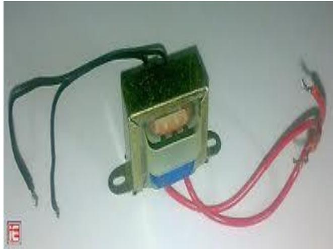
Gambar 2.9 Tranformator tegangan<sup>[5]</sup>
