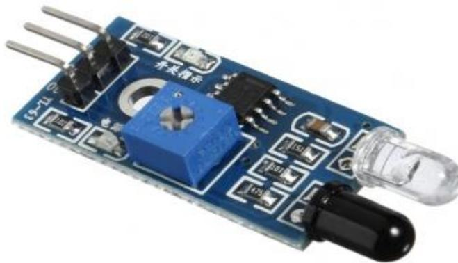
Gambar 2.12. Gambar Sensor Infrared Modul Arduino[2]
