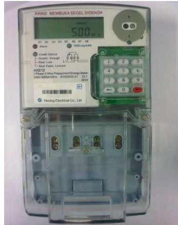
Gambar 2.2. kWh meter digital
