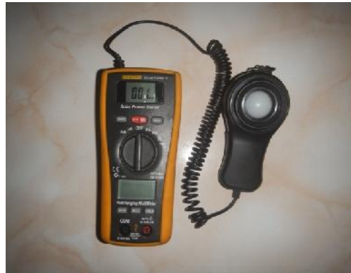
Gambar 3.5 Solar Power Meter .
