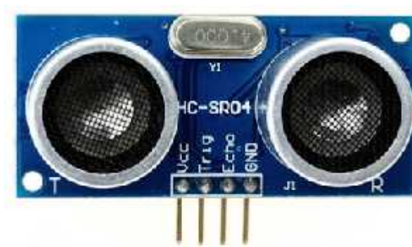
Gambar 2.8 Modul sensor ultrasonik HC-SR04
