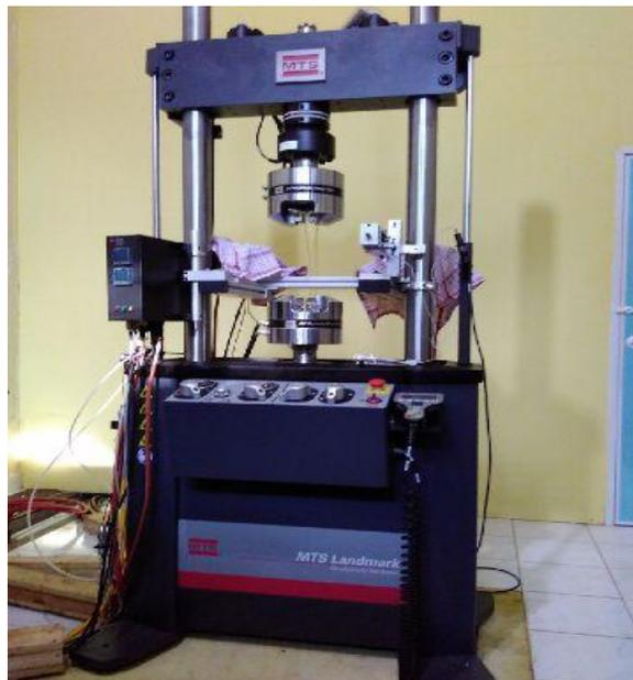
Gambar 3.2. Mesin MTS landmark 100 kN
