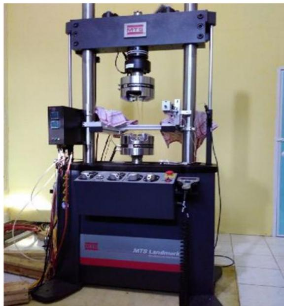
Gambar 3.2. Mesin MTS landmark 100 kN
