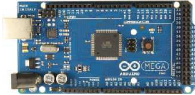
**Gambar 2. 1.** Board *Arduino Mega 2560 R3*
