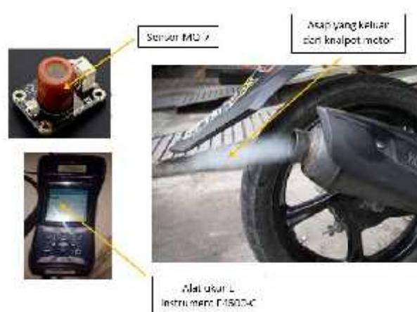
**Gambar 3. 14.** Kalibrasi Sensor MQ-7
