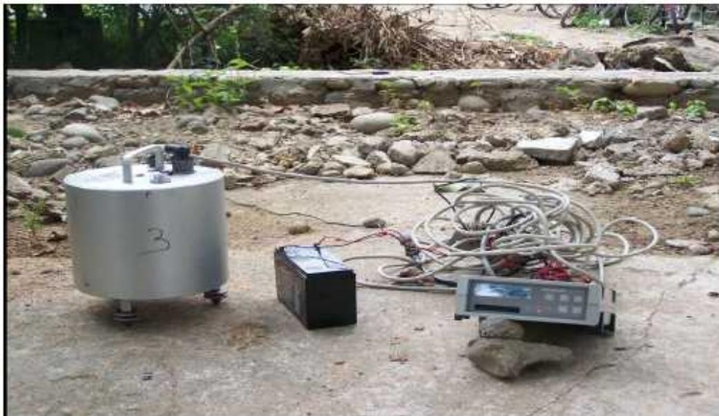
**Gambar 18.** Satu set peralatan mikrotremor (PVMBG)
