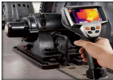
Gambar 19. Infrared thermography ( cfd-engineering.com )
