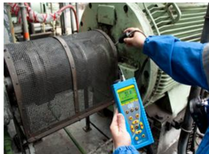
Gambar 18. Ultrasound condition monitoring (vibrasindo.com)
