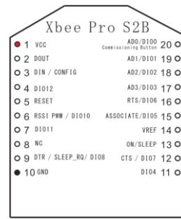
**Gambar 2.3 Konfigurasi Xbee Pro S2B**(Sumber : [http://www.inetclub.gr.jp/Total\\_collection\\_volume.htm](http://www.inetclub.gr.jp/Total_collection_volume.htm))
