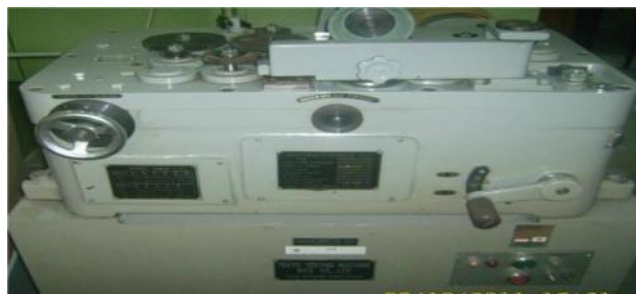
Gambar 12. Alat uji keausan Ogoshi high speed universal wear testing machine type OAT-U
