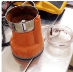
Gambar 3. Mesin *coffee grinder*
