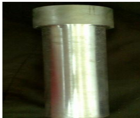
Gambar 13. Material Magnesium AZ31B ( Analysis of surface integrity in dry and cryogenic machining of AZ31B Mg Alloys , 2011)
