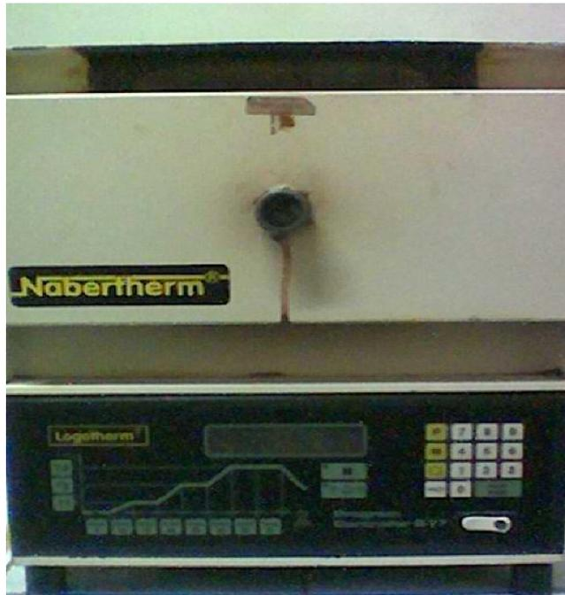
Gambar 3.1. Tungku sintering (*furnace*).
