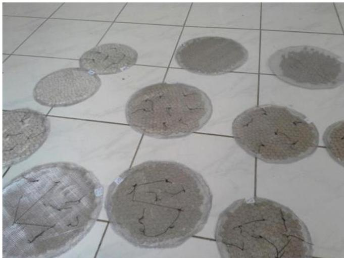
Gambar 26. *Filter zeolit-fly ash.*
