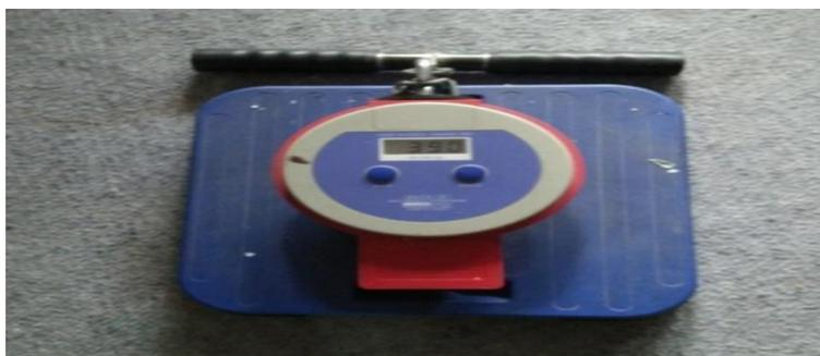
Gambar 9. *Back and Leg dynamometer*
