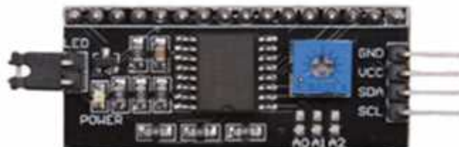
Gambar 2.8. Komunikasi I2C ( Inter-Integrated-Circuit )
