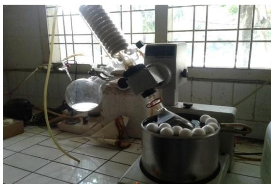
Gambar 7. Alat *Rotatory Evaporator*
