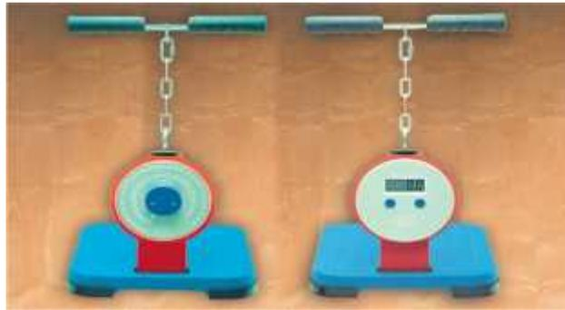
Gambar 6. *Leg Dynamometer*
