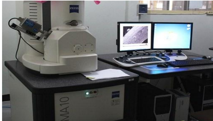
Gambar 19. Alat SEM EDX ( Scanning Electron Microscope ) di laboratorium F-MIPA Universitas Lampung
