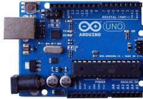
**Gambar 2.9** Arduino Uno (*Texas Instrumentation, 2016*)
