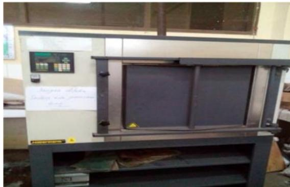
**Gambar 3.12.** *Furnace*, berfungsi proses *curing* komposit.
