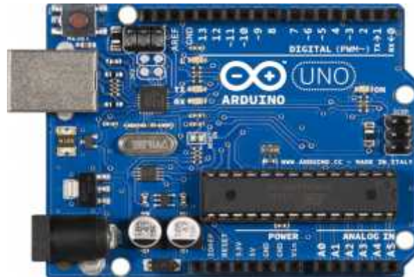
Gambar 4. Board Arduino UNO (Saputri, 2014).
