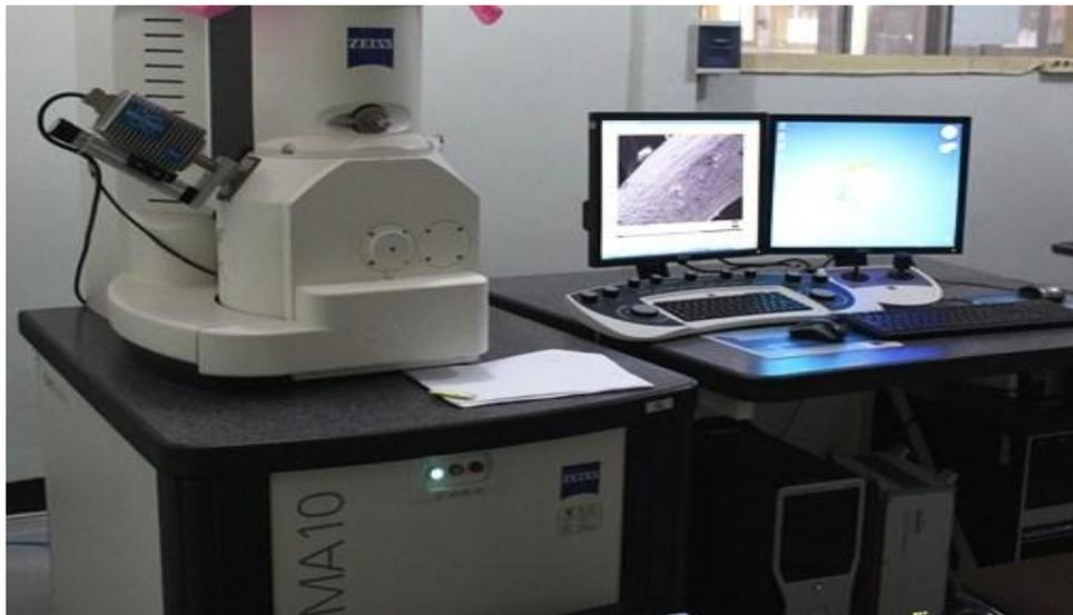
Gambar 3.4.Scanning Electron Microscope (SEM-EDX) ZEISS EVO® MA 10
