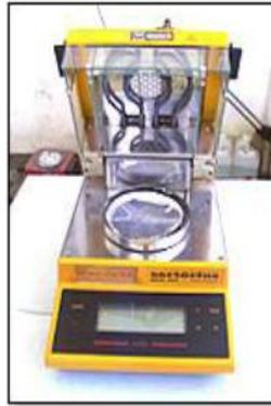
Gambar 6. *Moisture analyzer type MA 30* (Desiana dkk, 2012).
