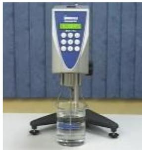
**Gambar 8.** Viskometer
