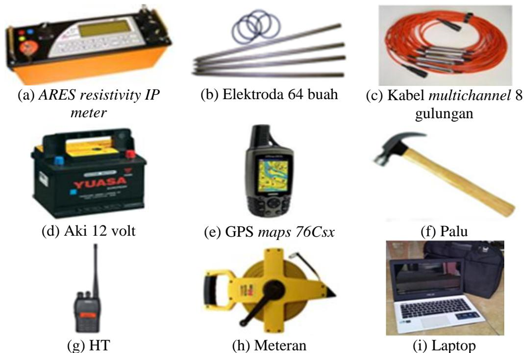
**Gambar 9.** (a) *ARES resistivity IP meter*, (b) Elektroda, (c) Kabel, (d) Aki, (e) GPS, (f) Palu, (g) HT, (h) Meteran, (i) Laptop
