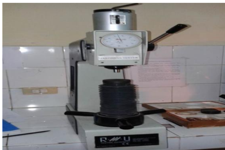
Gambar 10. Universal Hardness Tester
