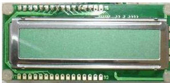
Gambar 2. 11. *Liquid Cristal Display* (LCD) 16 x 2 (Zain, 2013)
