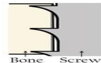
Gambar 11. Non-Self-Tapping Screws (Sumber: Gilley and Gold. 2006).
