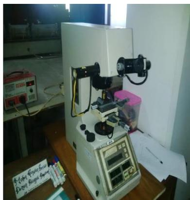
Gambar 14. Alat uji *Micro Hardness*
